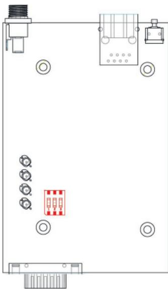
Remove the NPort P5150A's top cover and you will find DIP switches to adjust each serial port's pull-high, pull-low, and terminator. Do not use the 1 K $\Omega$  setting with RS-232 mode, as doing so will degrade the RS-232 signals and shorten the communications range.
