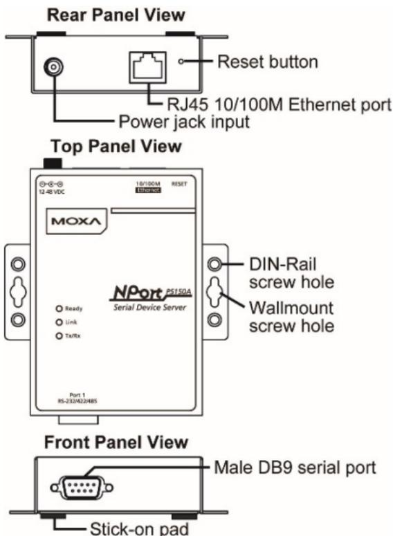
**Reset Button**—*Press and hold the Reset button for 5 seconds to load factory defaults:* Use a pointed object, such as a straightened paper clip or toothpick, to depress the reset button. This will cause the Ready LED to blink on and off. Once the Ready LED stops blinking (after about 5 seconds), release the reset button and the device server will start to load the factory defaults.
