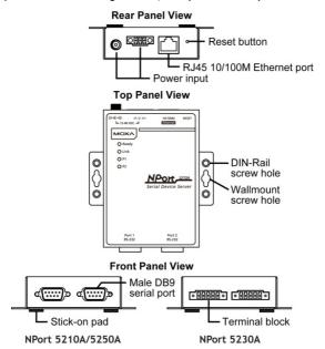
**Reset Button**—<u>Press and hold the Reset button for 5 seconds to load factory defaults:</u> Use a pointed object, such as a straightened paper clip
