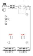
Remove the NPort 5230A/5250A's top cover and you will find DIP switches to adjust each serial port's pull-high, pull-low, and terminator. Do not use the 1  $\ensuremath{\mathrm{K}\Omega}$  setting with RS-232 mode, as doing so will degrade the RS-232 signals and shorten the communications range.
