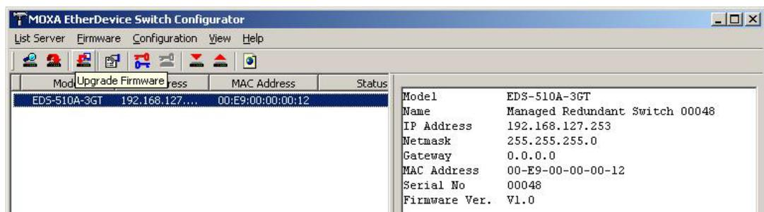
3. Click the **Upgrade Firmware** toolbar icon
