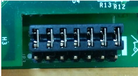
When the jumper is configured for one MAC mode, the ioPAC 8600 programmable controller will support the Ethernet Bypass function. In this case, you can connect the ioPAC 8600 using a daisy-chain architecture.
