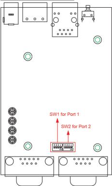
Pull High/low Resistors for the RS-485 Port
