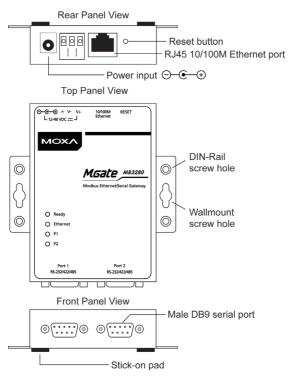
**Reset Button**—The reset button is used to load factory defaults. Using a pointed object such as a straightened paper clip to hold the reset button down for five seconds. Release the reset button when the Ready LED stops blinking in order to load the factory defaults.
