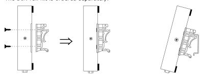
**Mounting on the wall:** Place two screws in the wall and slide the unit onto the screws as shown. The head of the screws should be 5 to 7 mm in diameter, the shaft should be 3 to 4 mm in diameter, and the length of the screws should be at least 10.5 mm. Leave about 2 mm of space between the head and the wall.
