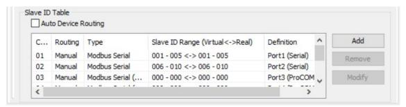
Select the first channel and click **Modify**. The Slave ID represents the Virtual ID recognized by the Modbus client/master.
