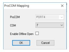
Once finishing configuring the COM port, click  $\mathbf{OK}$  and check if the COM port is changed successfully.
