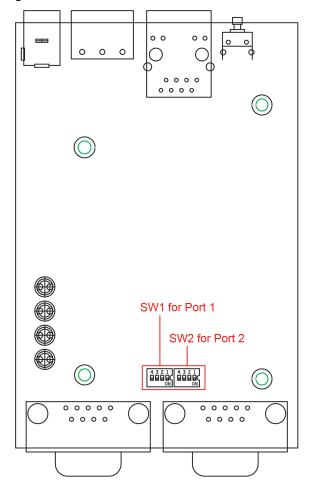
To access these switches, loosen the screws on both sides of the device and open the cover.
