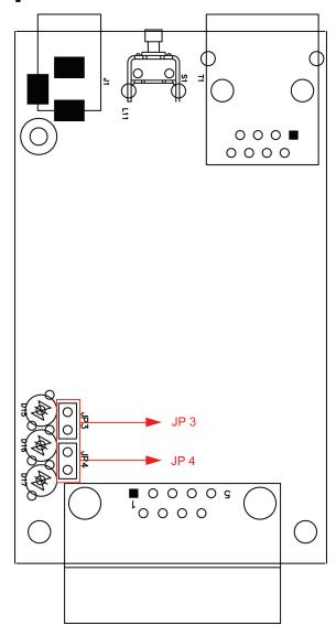
To access these jumpers, loosen the screws on both sides of the device and open the cover.
