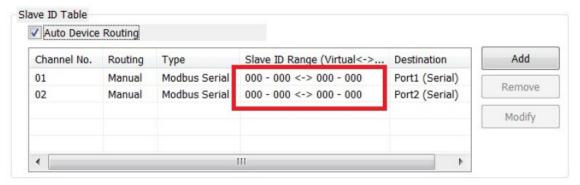
Users can only check the result of an auto-detect routing table through the web console.
