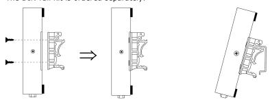
**Mounting on the wall:** Place two screws in the wall and slide the unit onto the screws as shown. The head of the screws should be 5 to 7 mm in diameter, the shaft should be 3 to 4 mm in diameter, and the length of the screws should be at least 10.5 mm. Leave about 2 mm of space between the head and the wall.
