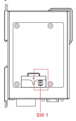
The DIP switches are beneath the DIP switch panel on the side of the unit.
