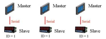
The MGate MB3000 can connect to each serial server/slave, so Ethernet SCADA clients/masters will be able to control them. However, since slave IDs cannot be repeated in a system, we will need to change the IDs of some of the servers/slaves to integrate them into a single network, as follows:
