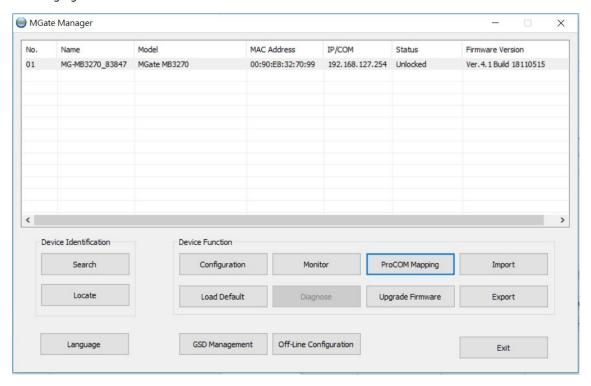
On the ProCOM mapping dialog box, you can map up to four ProCOM functions for each Modbus gateway to your PC's COM ports. The driver will generate virtual COM ports on your PC to connect to the selected MGate MB3x70 over the network.
