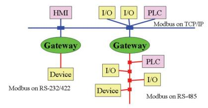
Ordinarily, Modbus TCP and Modbus ASCII/RTU cannot communicate with each other. However, with a Modbus gateway in between the Modbus serial network and the Modbus Ethernet network, TCP clients/masters can communicate with serial servers/slaves, and serial clients/masters can communicate with TCP servers/slaves.
