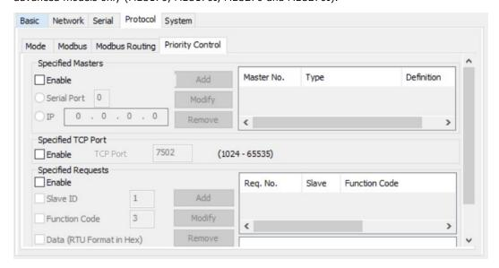
Priority control is designed for requests that are sent to Modbus RTU/ASCII servers/slaves. Since Modbus RTU/ASCII servers/slaves cannot handle multiple requests, the Modbus gateway must send each request individually and wait for the response before sending the next request. As requests stack up, the response time can suffer. This can cause problems for certain critical requests that require an immediate response.
