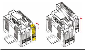
**NOTE** Electrical connections to the internal bus will be disconnected when the 45MR module is removed..
