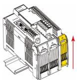
$\mbox{Step 2:}$  Push the top of the release tab to latch it, and then pull the module out.
