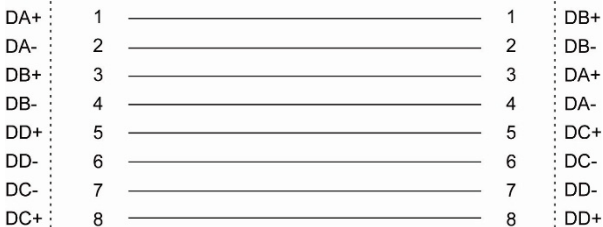
Straight-through Cable Wiring (MDI to MDI-X)
