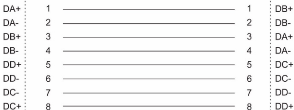
Straight-through Cable Wiring (MDI to MDI-X)
