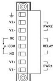
**STEP 1:** Insert the negative/positive DC wires into the V-/V+ terminals.
