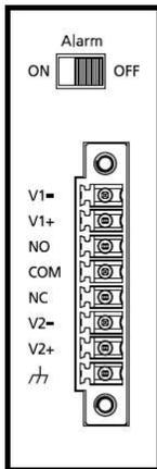
**RELAY:** The three middle contacts of the 8-contact terminal block connector are used to detect both power faults and port faults. The two wires attached to the fault contacts form an open circuit when:
