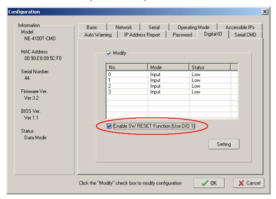
As indicated, the RESET command will be transmitted through GPIO1.
