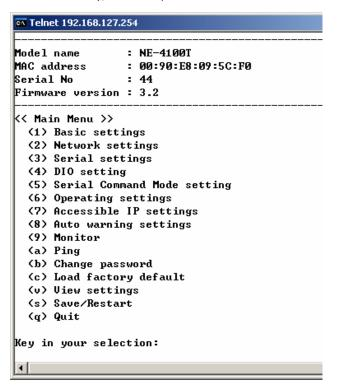
2. The Telnet Console is easy to use. To select an option, type the character next to the option and then press **Enter**. For example, type **5** to select **Serial Command Mode** setting.
