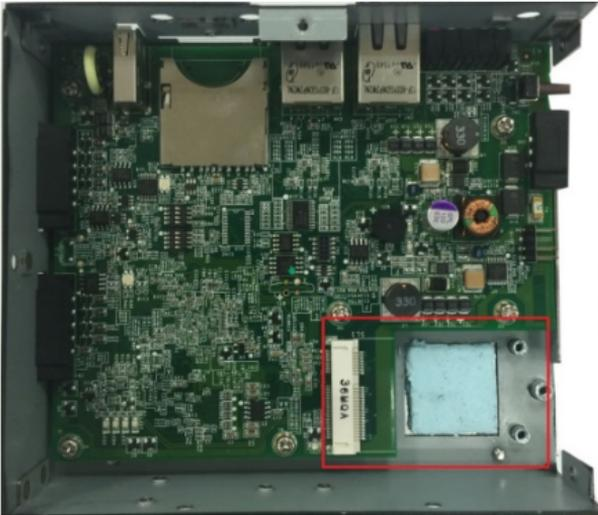
9. Remove the screw next to the socket and replace it with the bronze screw (in the package) as shown below:
