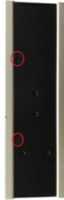
3. Remove the four screws on the silver cover on the right panel and remove the cover.
