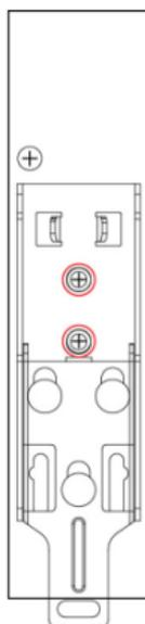
2. Pull down the bottom slider of the DIN-rail bracket located at the back of the unit
