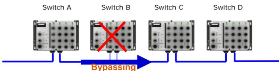
With the maximum segment length of category 5 twisted-pair cable being 100 meters, cable length must be considered when designing a network that utilizes this function. For example, the total length of the cables from Switch A to B and from B to C must be no more than 100 meters. This way, if the two adjacent nodes (switch B and C for example) encounter a power failure, there will be no stoppage, provided that the total length of the cables A-to-B, B-to-C, and C-to-D are no more than 100 meters.
