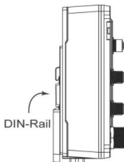
To remove the Moxa ToughNet Switch from the DIN-Rail, use a screwdriver to pull out the two spring-loaded brackets from the bottom until they are fixed in the “locked” position. Then reverse Step 3 and 4 above.
