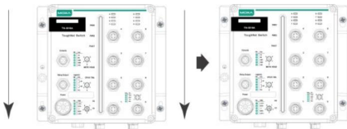
**NOTE** To provide greater protection from vibrations and shocks, use screws with shaft diameter between 6.0 mm and 7.0 mm, and fix the ToughNet switch onto the wall directly through the large opening of the keyhole-shaped apertures.
