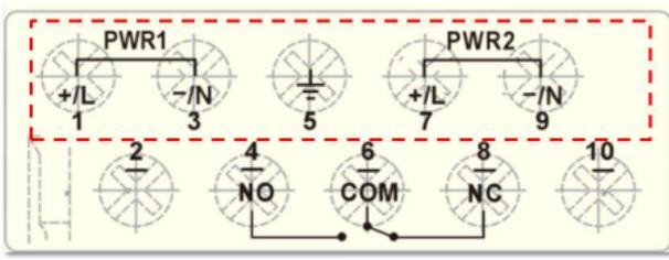
**STEP 1:** Insert the dual set positive/negative DC wires into PWR1 and PWR2 terminals (+ → pins 1, 7; - → pins 3, 9), or insert the L/N AC wires into PWR1 and PWR2 terminals (L → pins 1, 7; N → pins 3, 9).
