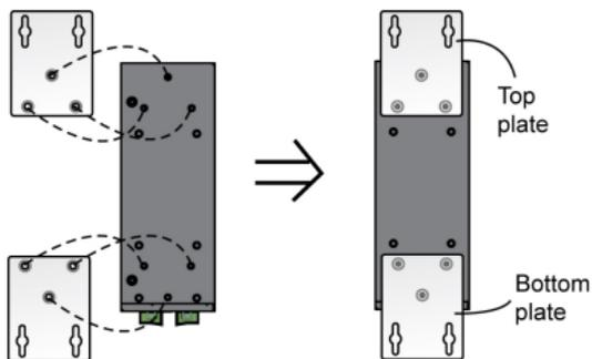
**STEP 2:** Mounting the PT-508 to a wall requires 4 screws. Use the PT-508, with wall mount plates attached, as a guide to mark the correct locations for the 4 screws. The heads of the screws should be less than 6.0 mm in diameter, and the shafts should be less than 3.5 mm in diameter, as shown on the right.
