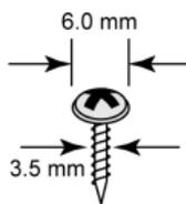
**NOTE** Test the screw's head and shank size by inserting the screw into one of the keyhole-shaped apertures of the wall mounting plates before screwing it into the wall.
