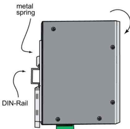
To remove the Moxa PT-508 switch from the DIN-Rail, use a screwdriver to push down the spring-loaded bracket until it locks in place, as shown in the following diagram. Next, rotate the bottom of the switch upwards and then remove the switch from the DIN-Rail.
