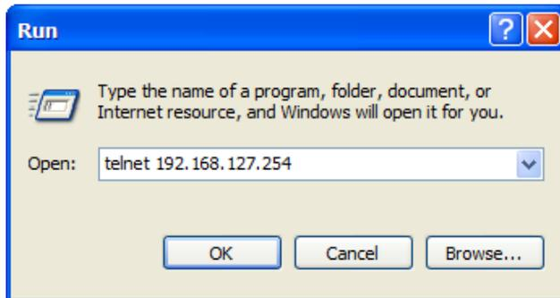
3. When the Telnet window opens, you will be prompted to input the Console password (the default username is **admin** and password is **moxa**; for the NPort 5100/5200/IA5000, it only requires the default password **moxa**); input the password and then press **Enter**.
