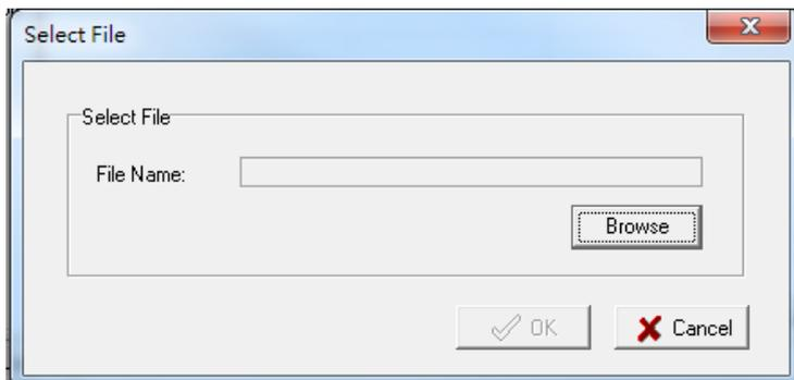
For the overall NPort 5000 Series with security enhanced firmware version, export configuration encryption will be based on the Pre-shared key defined in the NPort (default is empty password, and you may configure the password in **Configuration -> Configuration Pre-shared Key**). So when you are exporting the configuration file, you are only required to select the output file location. You may refer to page 2-21 for the security firmware version for your NPort.
