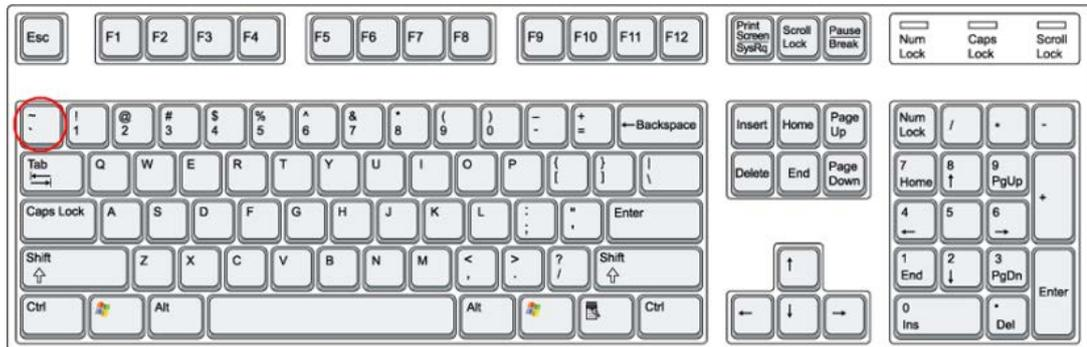
7. The NPort will automatically switch from data mode to console mode as it receives a continuous string of "`" characters.
