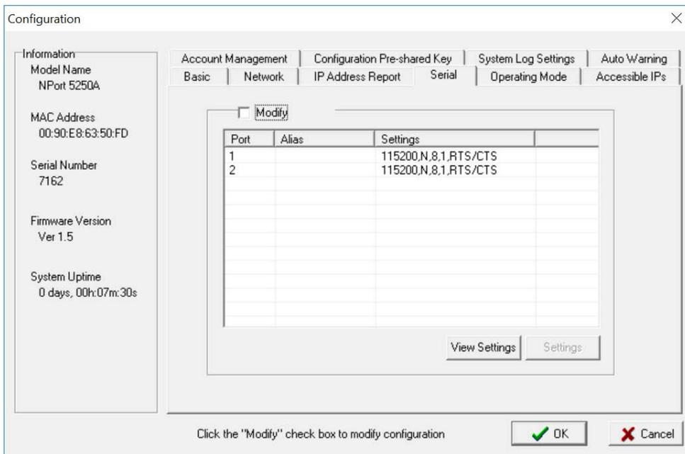
The serial communication parameters for each device port can be configured through NPort Administrator. Open your device server's configuration window, using the same method you used to configure network parameters. On the **Serial** screen, select the **Modify** check box and then select the device port that you wish to configure. Click **Settings** to configure the selected device port.
