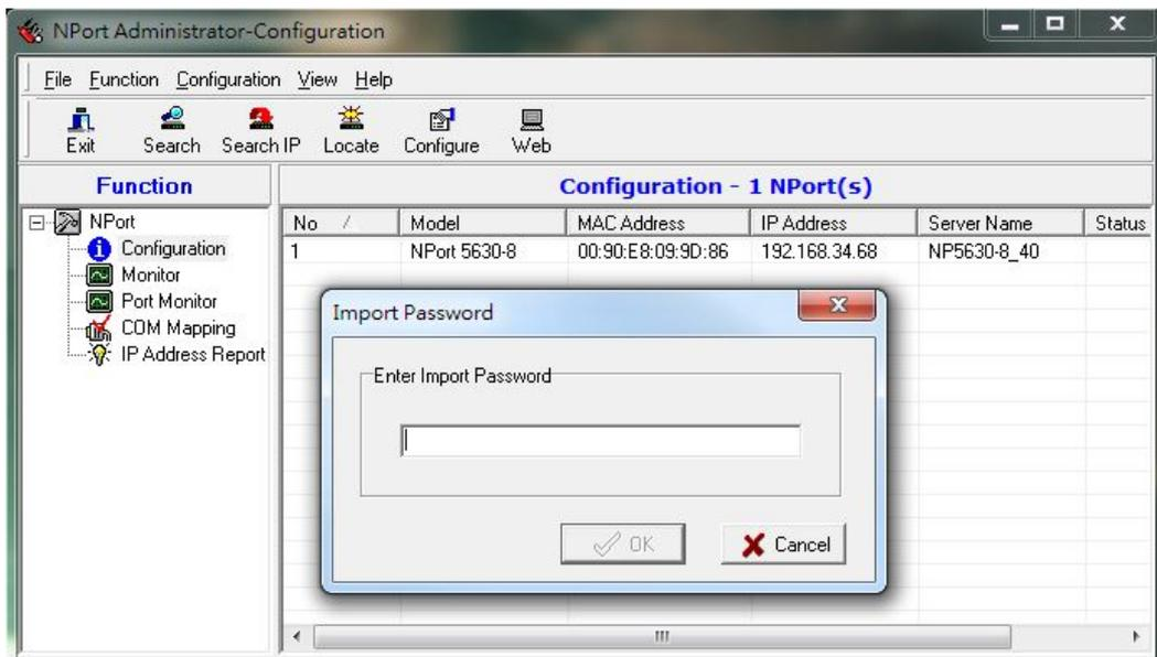
For the overall NPort 5000 Series with a security enhanced firmware version, importing configuration decryption will be based on the pre-shared key defined in the NPort. If the pre-shared key does not match, you will see an error dialogue box on the screen.
