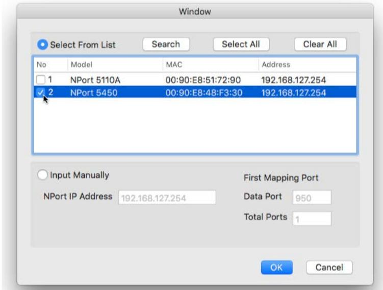
7. NPortConnect would auto assign the tty name and corresponding port number to the IP address of the selected NPort.
