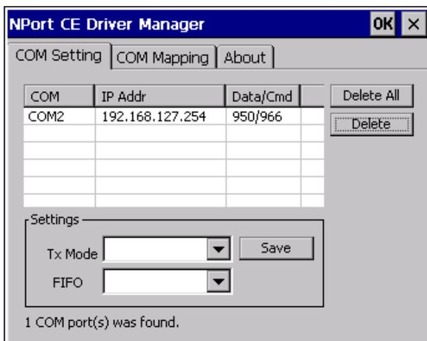
6. To configure the settings for a particular COM Port, select the row of the desired port, and then modify the setting in the "Settings" panel, as shown below.
