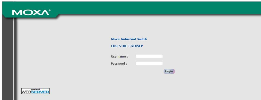
**NOTE** By default, the password assigned to the Moxa switch is **moxa**. Be sure to change the default password after you first log in to help keep your system secure.
