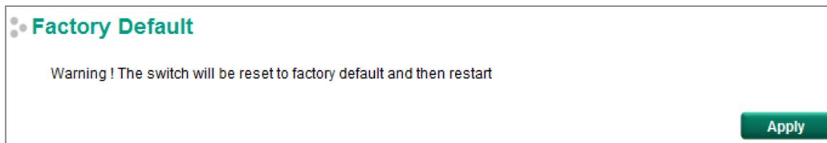
**NOTE** After restoring the factory default configuration, you will need to use the default network settings to re-establish the web or Telnet console connection with the Moxa switch.
