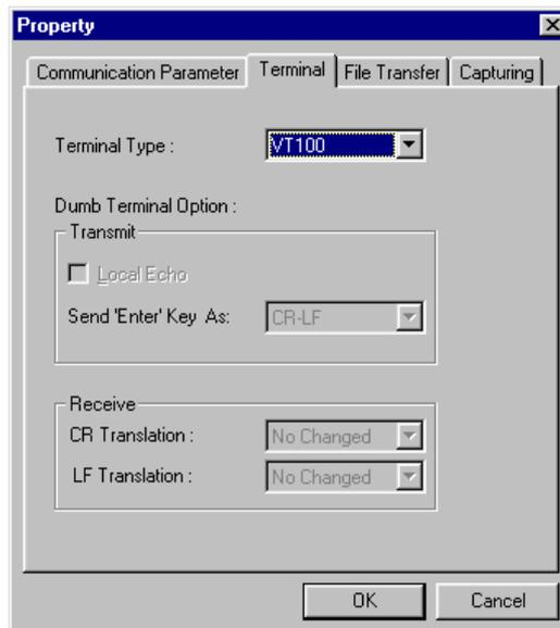
5. In the terminal window, the Moxa Ethernet extender switch will prompt you to select a terminal type. Enter **1** to select **ansi/vt100** and then press **Enter**.
