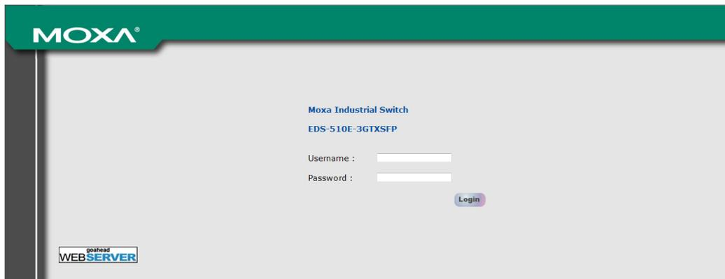
**NOTE** By default, the password assigned to the Moxa Ethernet extender switch is **moxa**. Be sure to change the default password after you first log in to help keep your system secure.
