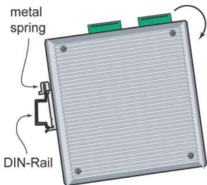
**STEP 2:** The DIN-Rail attachment unit will snap into place as shown in the following illustration.
