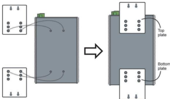
**STEP 2:** Mounting Moxa EDS-516A on the wall requires 4 screws. Use the EDS-516A, with wall mount plates attached, as a guide to mark the correct locations of the 4 screws. The heads of the screws should be less than 6.0 mm in diameter, and the shafts should be less than 3.5 mm in diameter, as shown by the figure on the right.
