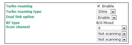
If you select to 100ms Turbo roaming, there are three roaming parameters, 802.11b/g (or a) roaming threshold, 802.11b/g (or a) roaming offset and 802.11b/g (or a) roaming alive would be shown as follows
