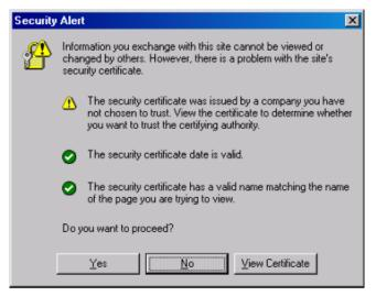
3. Select **Yes** to accept the certificate issued by Moxa IW and then enter the AWK-3121-RTG's web browser interface secured via HTTPS/SSL. (You can see the protocol in URL is **https**.) Then you can use the menu tree on the left side of the window to open the function pages to access each of AWK-3121-RTG's functions.
