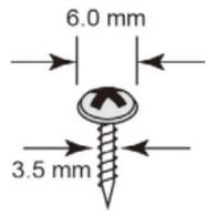
Do not screw the screws in all the way—leave a space of about 2 mm to allow room for sliding the wall mount panel between the wall and the screws.
