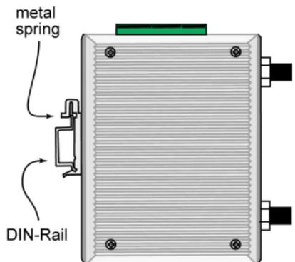
To remove the AWK-3121-M12-RTG from the DIN-Rail, simply reverse Steps 1 and 2.
